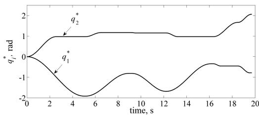
**Figure 3.** Input program signals for manipulator actuators
